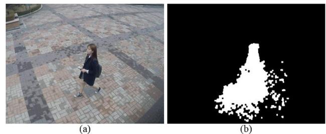
Fig. 1. Object Segmentation: (a) Input Image and (b) the Segmented Result of (a) Using Background Subtraction.
