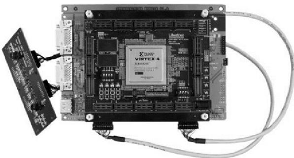
Fig. 3. Implemented real-time stereo vision system Based on FPGA
