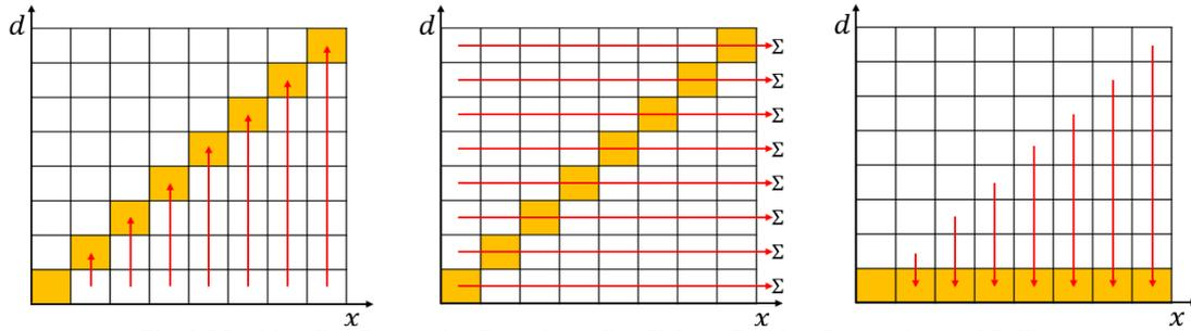
Fig. 4. Matching Cost Integration Procedure: Cost Volume Pushing, Integration, and Pulling
