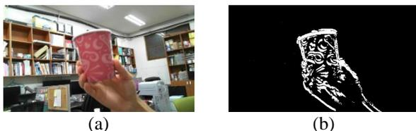
Fig. 3. The result of motion detection with the modified method by Mashak [5]: (a) an input video frame including a moving object, and (b) the detection result.
