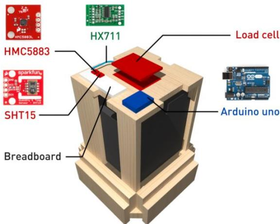
Figure 3. Connected sensors
