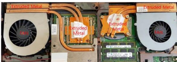
Fig. 4. Two fans and four pieces of extruded metal were used in the computer part.
